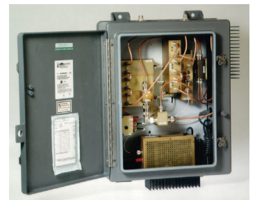
The TXRX Systems Signal Booster II
