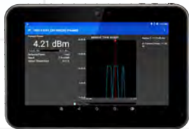
DIGITAL POWER METER DISPLAY
